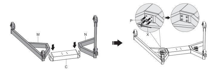
Attach the right base to the middle base and secure with screws(P). Repeat this step for the left base.
