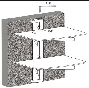
Attach the glass shelves to the glass holders using the screws and the plastic bushes.
