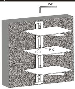
Attach the glass shelves to the glass holders using the screws and the plastic bushes.
