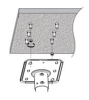
Attach the hex nuts to the expansion bolts corresponding to the keyhole pattern found on the ceiling plate. Do not overtighten and leave a small gap so the ceiling plate will slide into the keyhole slots.
